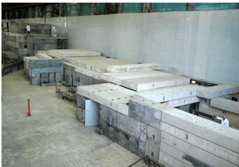
Figure 3: The TOF neutron spectrometer on the base of modified beam-stop
